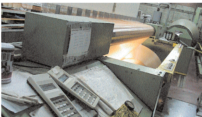
Each workstation is equipped with data collection terminals.
