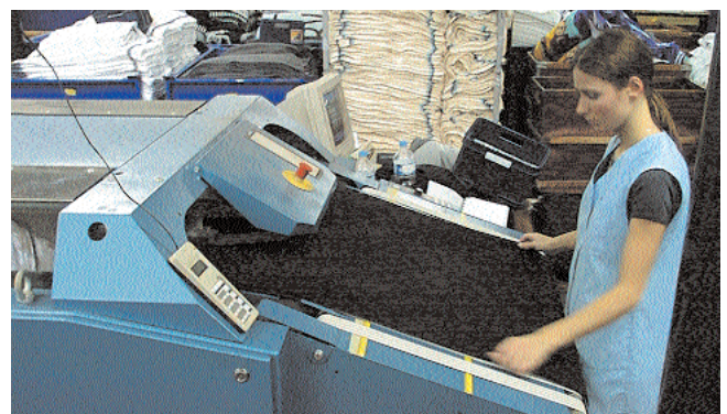
Using a simple dialogue the workers enter their personnel number, the order number, and the process they are doing at the start of the job.
